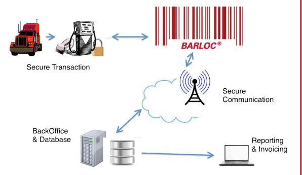
The BARLOC system is implemented at fuel islands at your truck yards. Integrated into the dispensers, the BARLOC system works with the dispenser technology to secure your fuel for consumption by authorized trucks.
